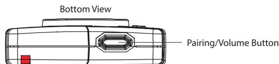
The volume has four settings. At each level, the camera beeps, providing you with a sample of the volume:
