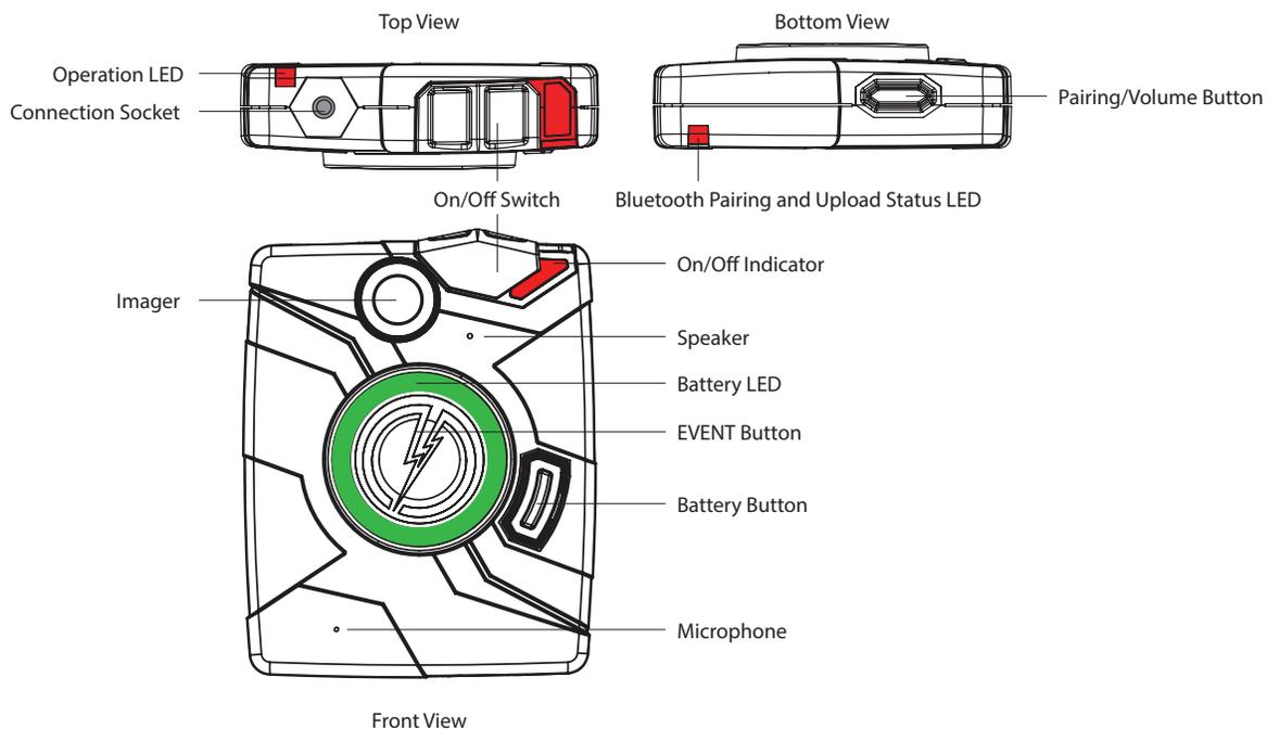
**1 Operation LED** – Shows the Axon Body camera's current operating mode:
